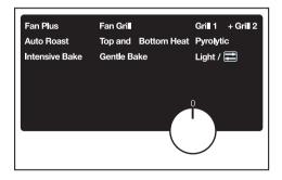
The programme selector is used for selecting your cooking function. It can be turned clockwise or anti-clockwise.
